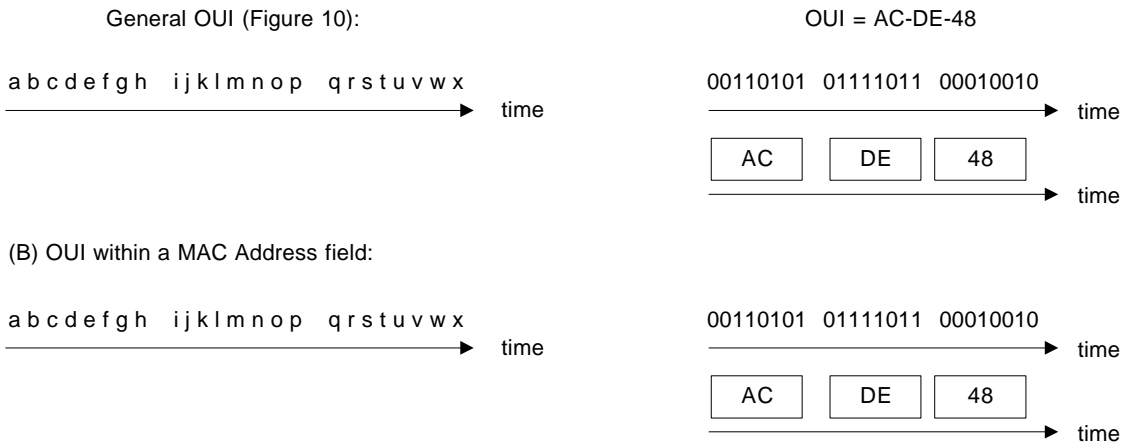
Figure 11—IEEE 802.3, etc., frame: Order of bit and octet transmission for an OUI
