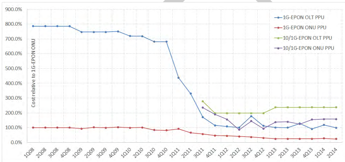
17 Figure 66: Relative Cost of 1G-EPON and 10/1G-EPON ONU and OLT Devices over Time
